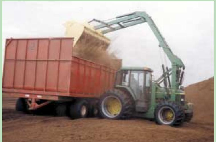
Loader has a 17-ft. lift height for loading into high-sized trucks.
