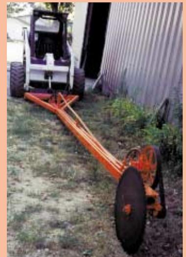
Blade is driven by a hydraulic motor that operates off loader's hydraulics.
