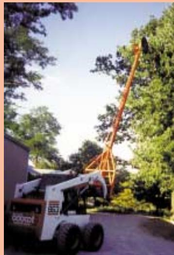
Skid loader-mounted saw can reach up to 25 ft. to trim overhanging branches.
