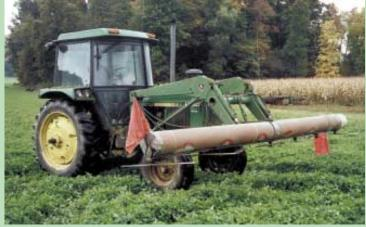
To keep debris from getting wrapped up in pulleys and drive belts, Graham made a protective shield out of 1-ft. dia. plastic pipe.
