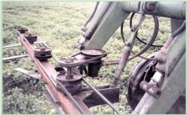
A single hydraulic motor positioned between loader arms drives all 7 blades at once.
