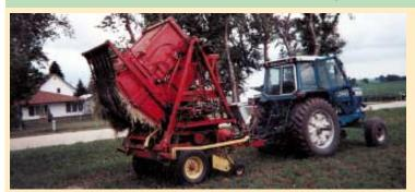
Agropack bale chamber swings back and forth, packing hay in accordion-like folds. Bales are rounded on one end to shed rain and snow.
