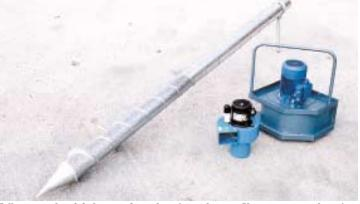
Hollow spear has 3-ft. long perforated section at bottom. You screw spear down into pile, then attach a blower to top of spear to blow cool air into grain.
