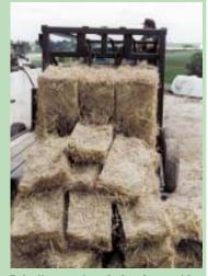
Bale slicer consists of a box frame with a ram or plunger at one end and knives at the other. Bale is pushed back through knives by plunger.
