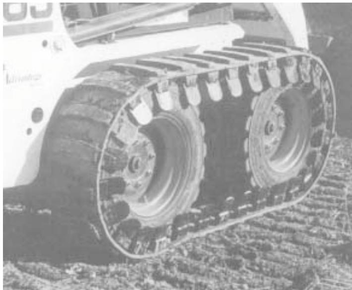
New track for skid loaders is fitted with steel alignment guides and replaceable polyurethane traction bars which can be replaced by unbolting them from the guides.
