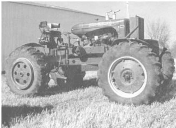
WC’s front axle is off a junked 1 1/2-ton 4-WD Dodge military vehicle. To make the front wheels, Landwehr cut the hubs off the axle and centered them on a couple of Deere manure spreader rims, fitting them with big 11.2 by 24-in. tires.
