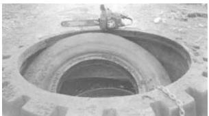
Bach converts large rubber earthmover tires which were given to him by a tire dealer. He uses a chain saw to cut bead off one side of tire.
