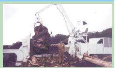
Splitter handles stumps up to 10 ft. in diameter and will split 6-ft. dia. logs up to 6 ft. long. The big splitter is so large it takes a lowbed heavy equipment trailer to haul it.
