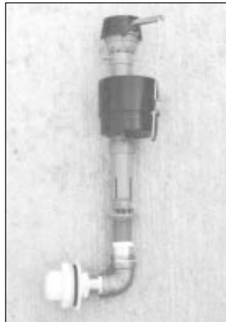
**Brass elbow with threaded fitting mounts inside tank and has a conventional flush box control and overflow outlet attached to it.**
