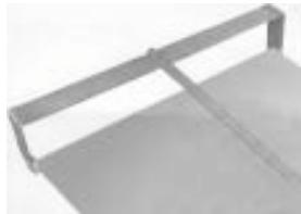
Slicer head rides on two 2-in. high poly wheels and has two cutting edges.
