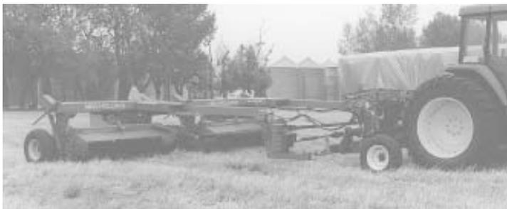
Hodge made the double-wide "reconditioner" by removing the cutterbars from two mower conditioners and hitching them together.
