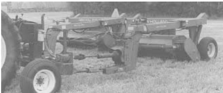
A pto-driven hydraulic pump drives two 50 hp. orbit motors which power the conditioner rollers on both units.
