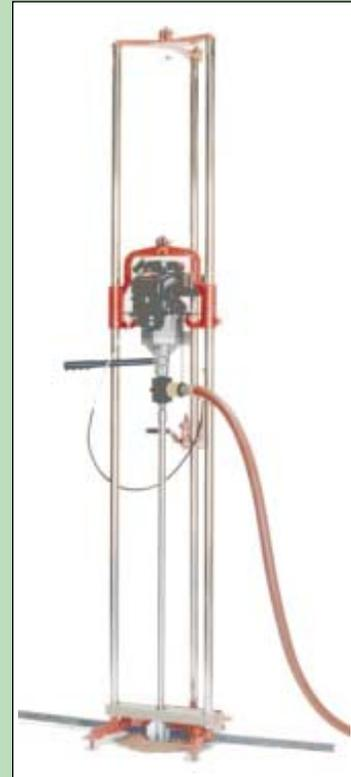
**Drill uses water and a "mud pump" that carries water and dirt away from hole. It can drill up to a 6-in. dia. hole.**
