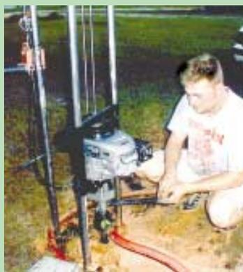
**HydraDrill is powered by a 4 or 6 hp 4-cycle single cylinder engine with a clutch and an 18:1 gearbox that turns the drill at about 170 rpm's.**
