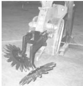
**Spoked wheels are staggered and set at a 50 degree angle.**
