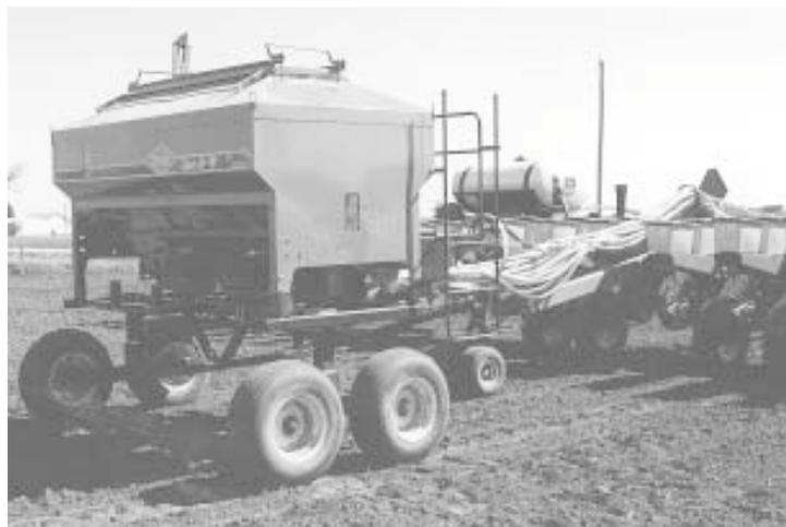
**Gandy system pneumatically delivers seed from a tow-behind bulk hopper to the individual row hoppers on planters.**
