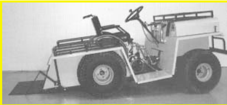
"Shuttlebug" has a ramp on back that's raised or lowered hydraulically for wheelchair access. It has three cargo racks that can haul up to 500 lbs.
