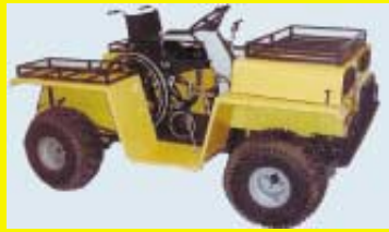
All functions on the machine are controlled by a single joystick.
