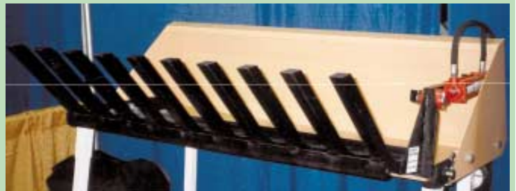
Rock picker slips over lip of existing bucket and bolts onto each side. Teeth are moved back and forth by a hydraulic cylinder that bolts onto back side of bucket.
