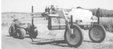
Power Roll's hydraulic-powered rotating rollers aggressively apply chemical to tall-growing weeds.
