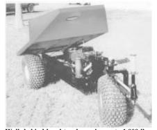
Walk-behind hand truck carries up to 1,000 lbs. of cargo and is controlled by a handle on front.
