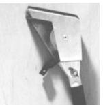
By loosening a wing nut, the head can be opened up like a clam in order to replace the tape roll.
