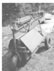
Splitter rides on three 14-in. wheels and is equipped with a four-way wedge for splitting big logs.
