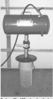
To clean a filter, Miller places it on the shop floor and sets the tank on top of it with a sheet metal circle over the filter. He then opens a valve to release air pressure.
