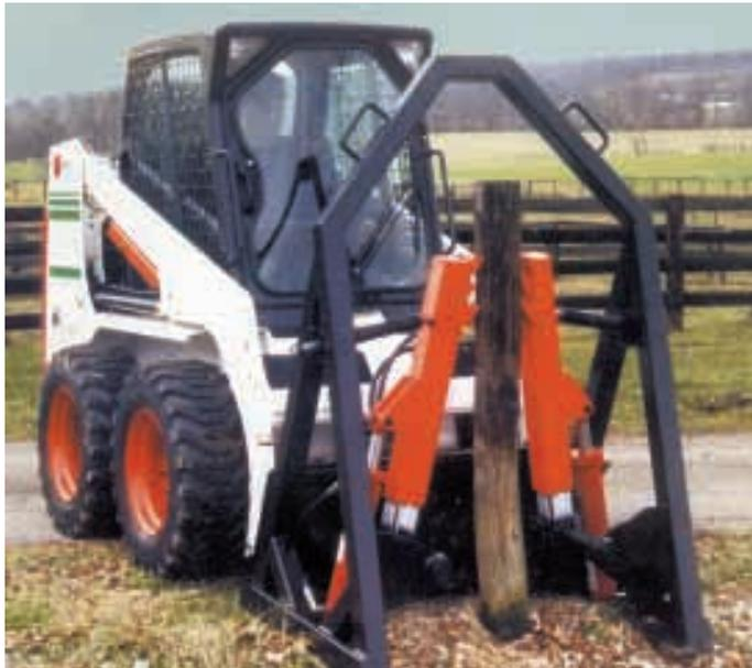
Post puller uses a pair of angled “tooth bars” to bite into post before pulling it out of the ground.
