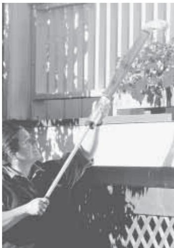
RainStick lets you water hanging plants or plants on high ledges. To use the unit you simply push on a plunger, which forces water out a curved nozzle.
