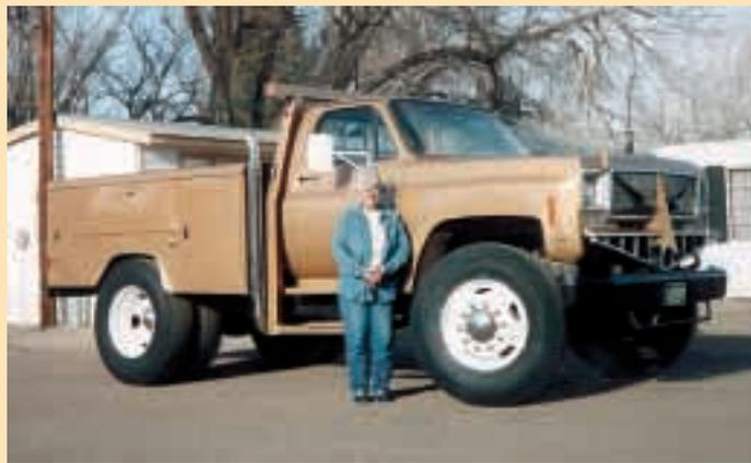
Bill Swets cut the cab and utility bed off his Chevy 3/4-ton pickup and mounted them on the frame and running gear of a school bus. Big pickup stands 7 ft. 10 in. tall.
