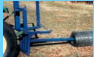
Unit tips down to ground to pick up fence roll and then raises it up.
