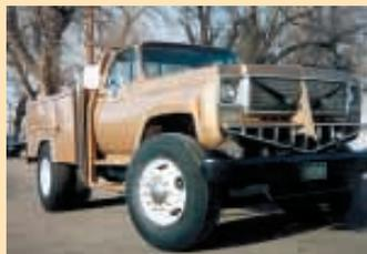
Pickup is powered by bus's original 366 cu. in., 250 hp engine.
