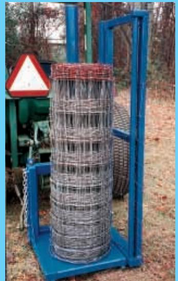
Fence Caddy allows one person to install fencing using a tractor. It picks up the roll, unrolls the wire, and stretches it. Fencing is fed out through a locking device that pulls it taut while you fasten it to your posts.
