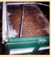
My new truck-mounted grain sampler makes it easy to collect an accurate sample from each truck load of grain. It consists of a 1 1/2-in. dia. pipe that runs diagonally about 2 ft. off the floor of the box from front to back. There are a series of 1-in. dia. holes spaced 1 ft. apart in the top part of the pipe. As grain is loaded into the truck it fills a couple inches of
