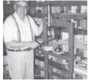
When he built this small hydraulic press, Clifford Brandenburger figured out a way to mount a 1 1/2-ton hydraulic jack upside down, resulting in a better view.
