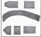
Chrome alloy liner bolts inside the blower chute. It consists of 6 1/2-in. wide overlapping sections that vary in length and shape, depending on chopper brand and model.
