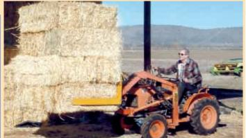
Designed specifically for utility tractors, "Mighty Mini Clamp" mounts on a front-end loader and can move large stacks of small square bales, as well as other materials
