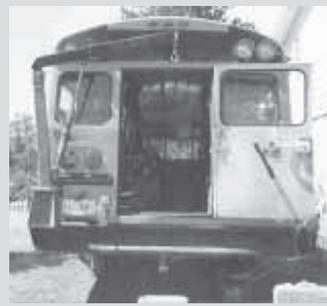
**Hand-cranked cherry picker mounts on bus's rear bumper, allowing Conlee to lift objects through rear emergency door.**
