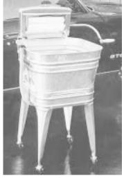
Hand-operated wringer uses two rubber rollers to squeeze water out of towels. S&H.
