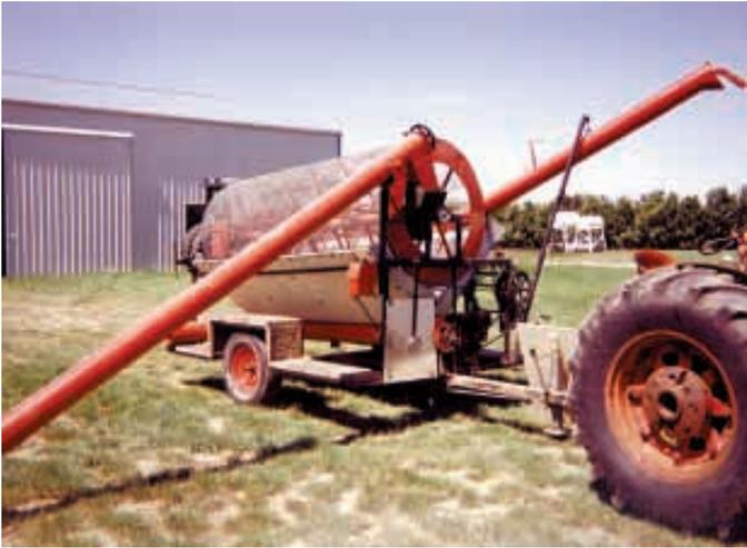
Seed cleaner measures 4 ft. in dia., 9 ft. long and is equipped with a pair of augers for loading and unloading.
