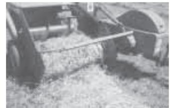
Bilodeau started with an IH 46 small square baler. He removed the baler's flywheel and cut off the bale chamber, and made an opening in back of baler for hay to flow through.
