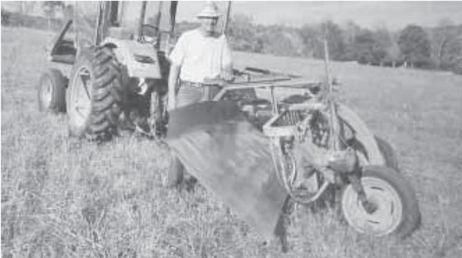
A 3-ft. wide tray mounts on front of Gannon's New Holland 256 basket rake, about 6 in. off the ground. When rake teeth pick up windrow to roll it, the tray catches it and slides the hay off the back onto drier ground.
