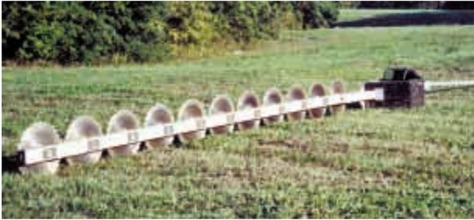
Helicopter saw consists of eleven 24-in. dia. circular saw blades attached to a 40-ft. long aluminum bar. Blades are belt-driven by a gas engine that mounts at one end of bar.
