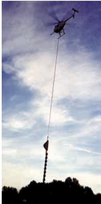
The 40-ft. long bar hooks to a steel cable suspended from helicopter. All operations are controlled by the pilot.
