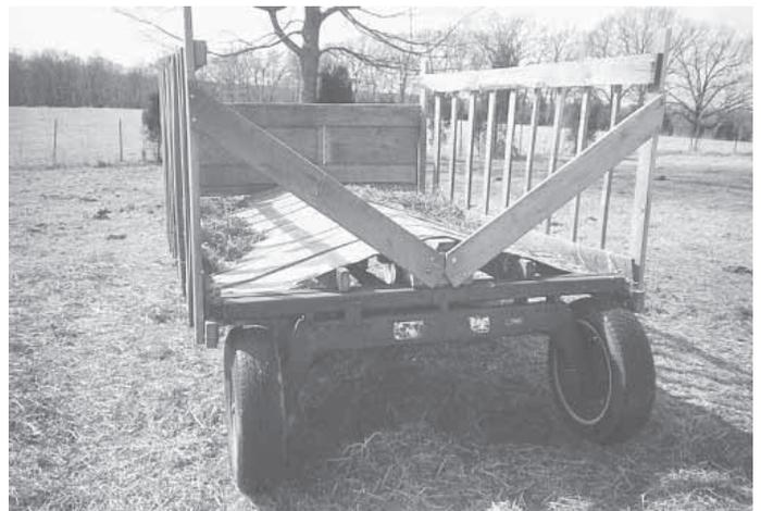
**To convert the wagon, the Weinerts built a bulkhead at one end and made wooden feed panels with uprights on 14-in. centers along both sides.**
