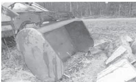
**Brackets that originally attached to legs of tank, are used to secure tank to loader arms.**
