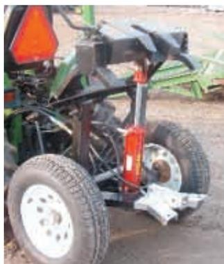
Hydraulic-powered dolly consists of a heavy-duty 2-wheel axle assembly that connects to 3-pt hitch on tractor. Works with 4-wheel drive tractor.
