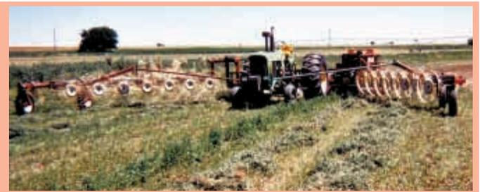
Twin balers and rakes mount at either end of double toolbar, gathering four windrows into two.
