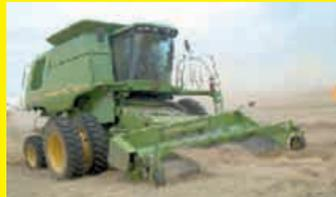
We recently introduced a new sidehill leveling system for Deere STS combines. The 2970S system is engineered as a bolt-on system that allows it to be installed on both new and used Deere STS combines. The 18 percent leveling capability is fully automated and delivers smooth, powerful leveling performance. An innovative undercarriage design keeps the tread face of the tire flat on the ground during leveling and can accommodate either single or dual drive tires.
