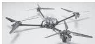
Radio-controlled helicopter measures 28 in. square and is fitted with a lightweight video camera.
