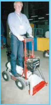
New 4-WD motorized nozzle cart supports a removable snout on front that hooks up to the hose on your grain vac. Operator uses hand controls to drive it around while standing on the unit. Eliminates the need to lift heavy grain vac hoses to clean grain out of a bin or quonset.
