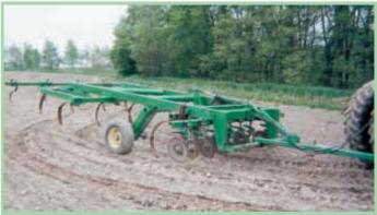
Using parts off an old tandem disk, Jeff Sebasty lengthened his 14-ft. chisel plow, increasing the spacing between the three chisel gangs to give crop residue more space to flow through.
