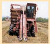
A grain elevator was converted to fit front of machine to pick up bales.
