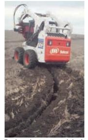
Trencher can be set at a steep vertical angle that allows it to turn sharply while digging. Auger's pull dirt away from trench.
