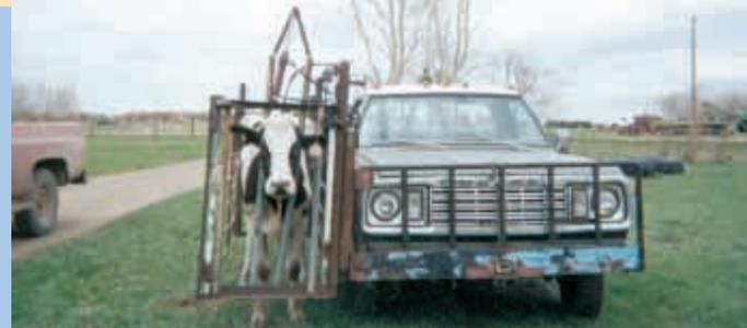
Chute mounts on passenger side of Dodge 1/2-ton 4-WD pickup. Both the headgate and swinging panel operate hydraulically.
