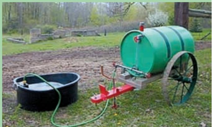
Water wagon was built out of a plastic 50-gal. drum and an old two-wheeled trailer.
