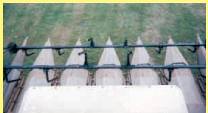
Both reels have big fingers, made of bent round tubing, over each row.
