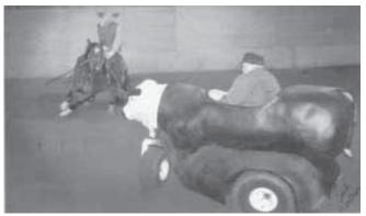
Mechanical bull has a fiberglass body that looks like a steer. Rider uses a pair of levers to control speed and steering. \$16,500.
