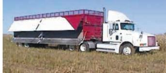
Trailer has an inverted "V" floor that's angled at 50 degrees and two independent sets of side doors. Upper door is hinged at top and opens hydraulically.
