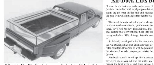
Unit consists of four 12-in. high aluminum panels that bolt to top of bed rails. "Lets you haul bigger, bulkier loads than you can with a cargo cap or tarp," says John Chechuck.
