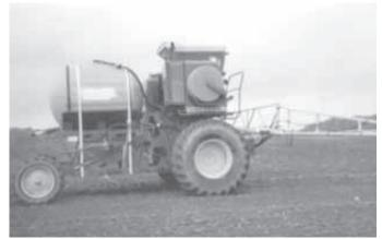
After the feederhouse auger on his Deere 7700 combine got damaged, Steve Kizer converted the combine into a self-propelled sprayer. It's equipped with a 60-ft. boom.
