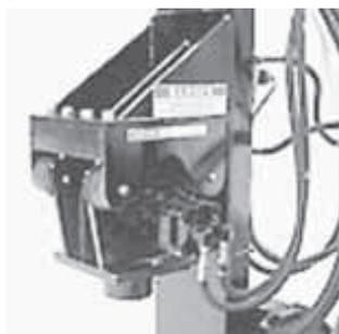
Unit is driven by a hydraulic motor that operates off skid loader's hydraulics. Steel cup lowers over top of post so it can't move or deflect sideways.
