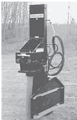
"Vibrating" post driver uses steady down pressure and quick taps to install posts.
