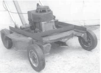
Krenzel cut off the front part of an old push mower, then replaced the original blade with a flat one fitted with sickle mow er knife sections.
