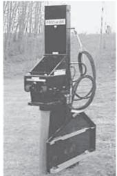
"Vibrating" post driver uses steady down pressure and quick taps to install posts.
