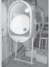
Rich DeVries built this stationary sand blasting cabinet out of a 250-gal. fuel tank and scrap steel.
