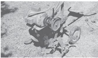
Electric motor, with pulley attached, bolts on in place of rototiller's original gas en-
