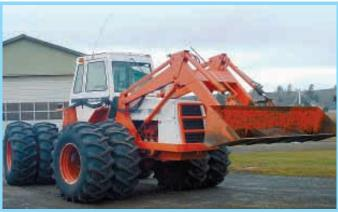
Ron Kile cut this tractor in half to convert it to articulated steering. He built a frontend loader to fit the big tractor
