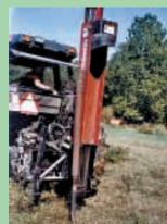
Bale spear welded to pipe punches holes in hard ground for fence posts.
