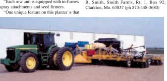
Planter's fitted with a Yetter Seed Jet that loads and unloads the seed hopper.
