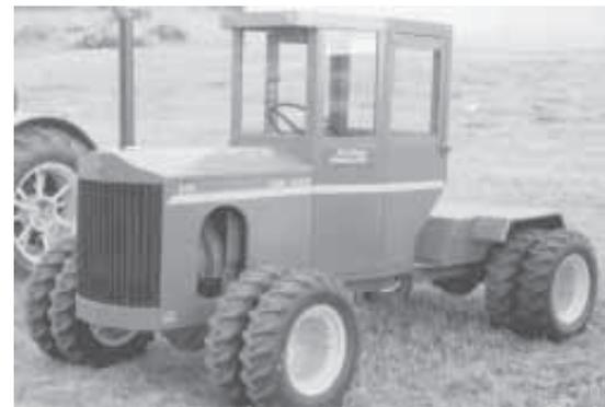
Miniature Deere 2418 articulated tractor is powered by an 18 hp, 2-cyl. LUC gas engine off an old Deere A12 combine.
