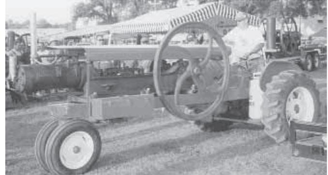
Hunter mounted a Thomas "half-breed" oil field engine on a stretched-out 1936 Allis WC tractor. Note big 4-ft. dia. flywheel on one side and water cylinder on front.
