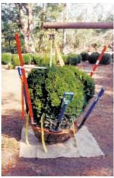
Low-cost shrub mover uses a bunch of ordinary hand-held shovels held together by metal bars and nylon straps. It hangs from a 12-ft. "boom" that attaches to his loader tractor.
