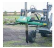
When operator lifts loader and tips it back, edge of gate bites into side of post to pull it out of ground.
