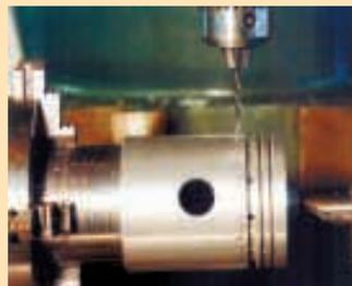
Once the piston has been cast, Chastain completes the finishing work.
