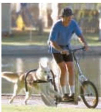
Adult-sized scooter has curved rear outrigger made from bicycle tubing, to which dog can be harnessed. A second or third outrigger can be added.
